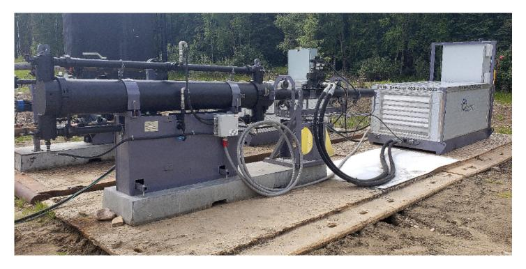
The MPTP is specifically designed for use at a satellite or header where production from multiple wells is collected. The resulting drop in flowline and casing annulus pressure allows the wells feeding into the MPTP to produce more.
